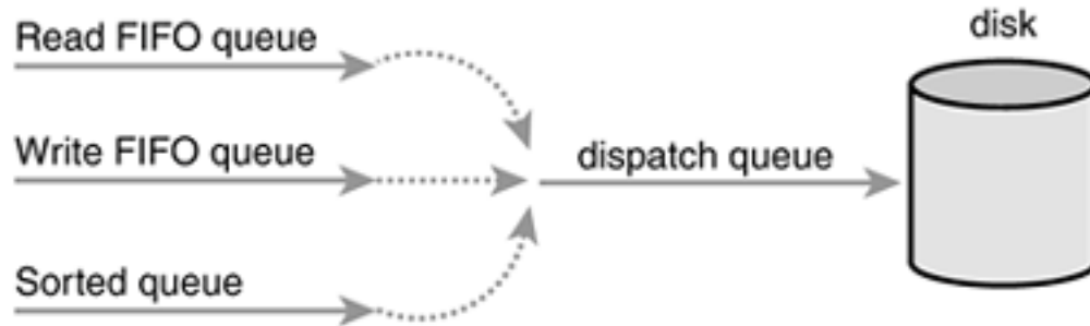
Figure 13.3. The three queues of the Deadline I/O scheduler.
