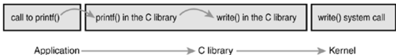
Figure 5.1. The relationship between applications, the C library, and the kernel with a call to printf() .
